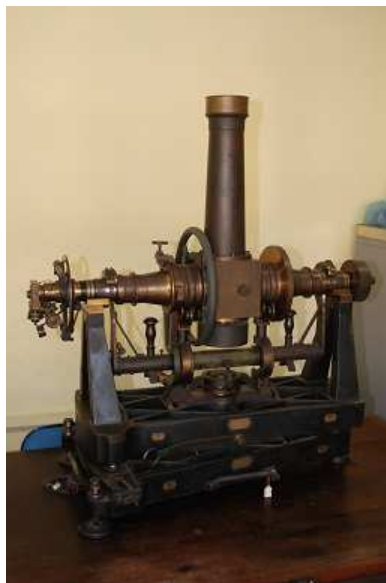
FIG. 1 - A photo of the Bamberg Meridian Circle.
