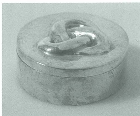
Fig. 8 Silver box after treatment in pure hydrogen plasma for 55 minutes, the maximum temperature being 93° C. The tarnish is removed.
