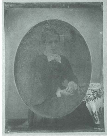
Fig. 6 The same daguerreotype after 54 minutes hydrogen plasma treatment, at a maximum temperature of 85° C.
