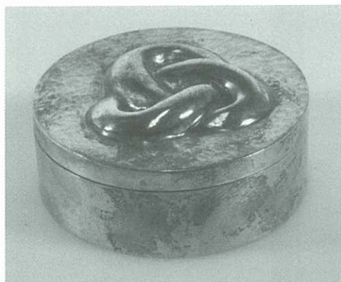
Fig. 7 Silver box before plasma reduction showing tarnished areas including fingerprints.
