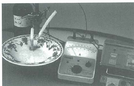
Fig. 3 Cleaning of iron stains on a ceramic recovered from the wreck of the Titanic (credit EDF-Valectra).
