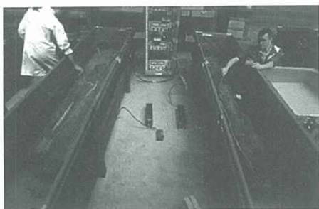
Fig. 2 Treatment of two of the bronze cannons recovered from the wreck of the San Diego (credit ART-Métal).
