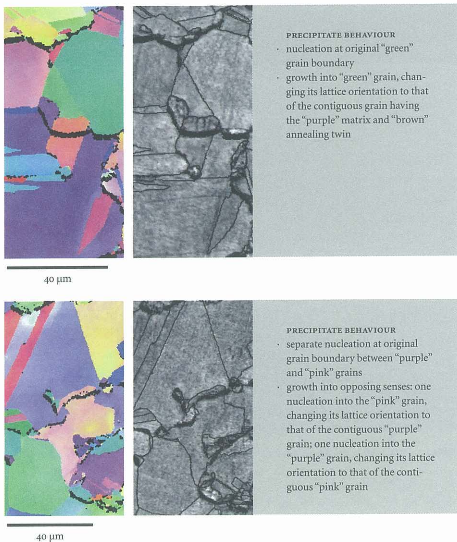
Fig. 4 Details of precipitate nucleation and growth in sample 366.
