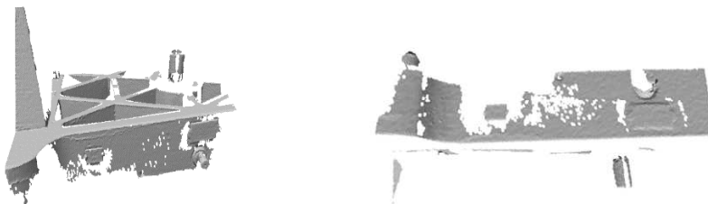
FIG. 4 - Two registers from the scanner. Note how there are many missing parts and holes due to the material dark color. The laser is also unable to reach inside the base's apertures.
