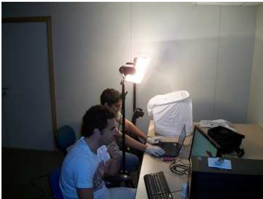
FIG. 8 - A photography session using the small diffuse white box and two light sources.
