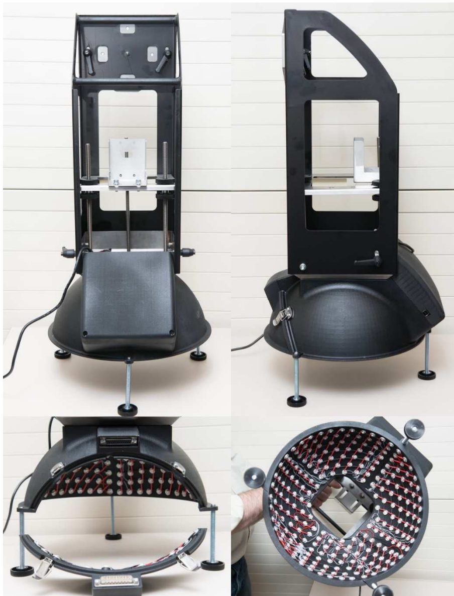
FIG. 1 - The construction of the Microdome with the rigid superstructure to fit the camera and lens combination. The structure can be mounted on standard photographic equipment such as a tripod or studio stand, allowing the user to position the Microdome in the desired angle. The MS Microdome has the exact same setup. (©RICH project, KU Leuven).
