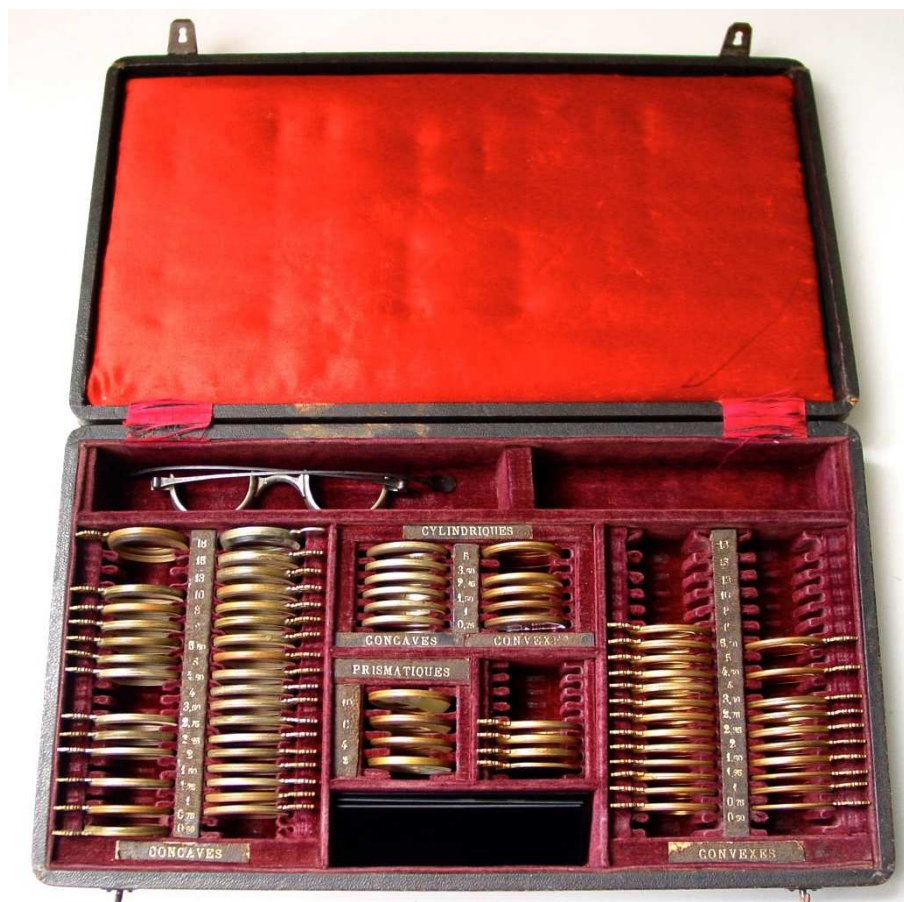
FIG. 19 - Optician's trial set of lenses (Physics collection of the Museum of Science, Inv. 000374).
