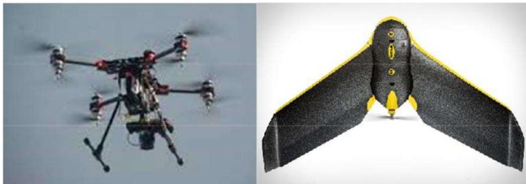
Figure 1: (a) Multi-rotor UAV and (b) Fixed-Wing UAV (SenseFly eBee)
