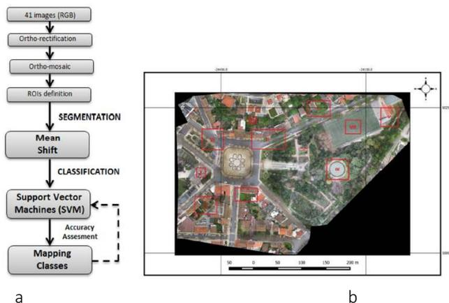
Figure 2: (a) Workflow of the methodology employed; (b) Study area (ortho-mosaic) with the 10 ROIs marked
