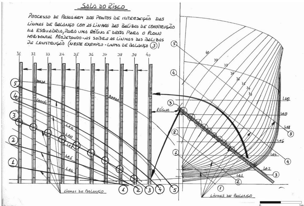
Fig. 3.6. Horizontal projection of balance lines
