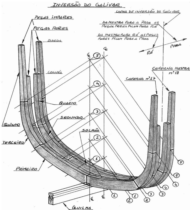
Fig. 3.14. Reversing the position of the even parts with the odd parts in the master frame
