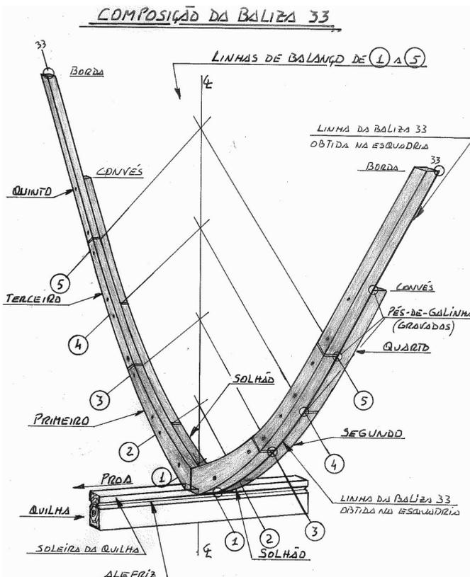
Fig. 3.12. Design of frame 33 in perspective
