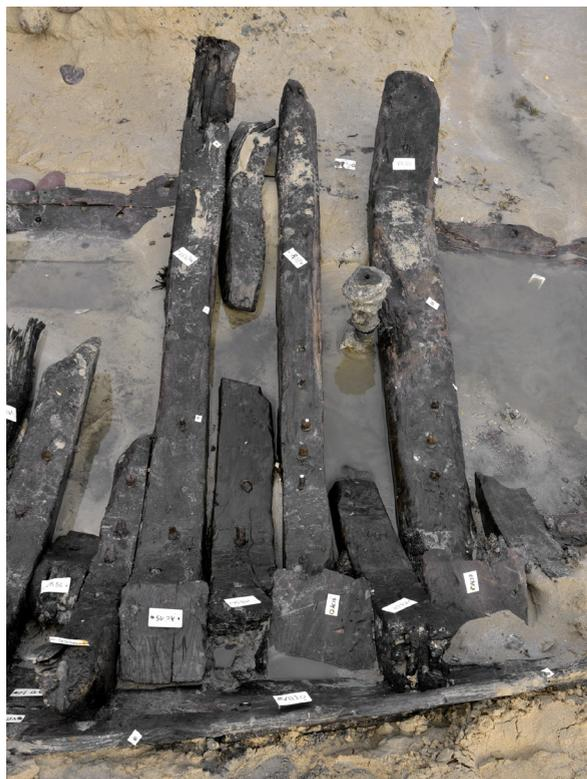
Fig. 1.11. Obliquely worked lower extremities of the futtocks; the direction of the bevel is reversed
