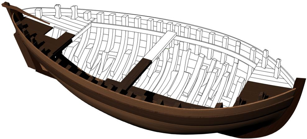
Fig. 1.17. 3D reconstruction of the architectural structure
