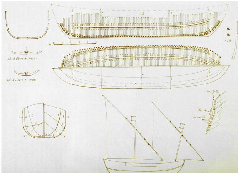
Fig. 2.22. Drawings and graphic reconstruction of the *Contarina 1*
