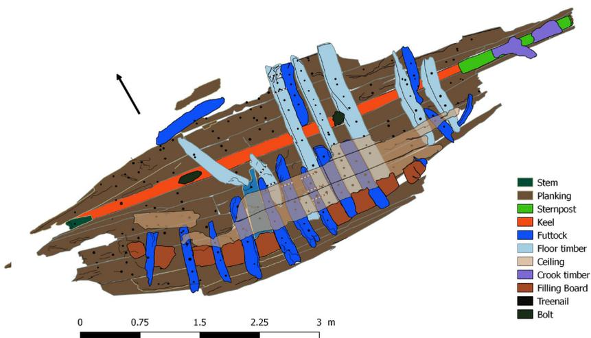
Fig. 1.10. Planimetric view of the architectural remains
