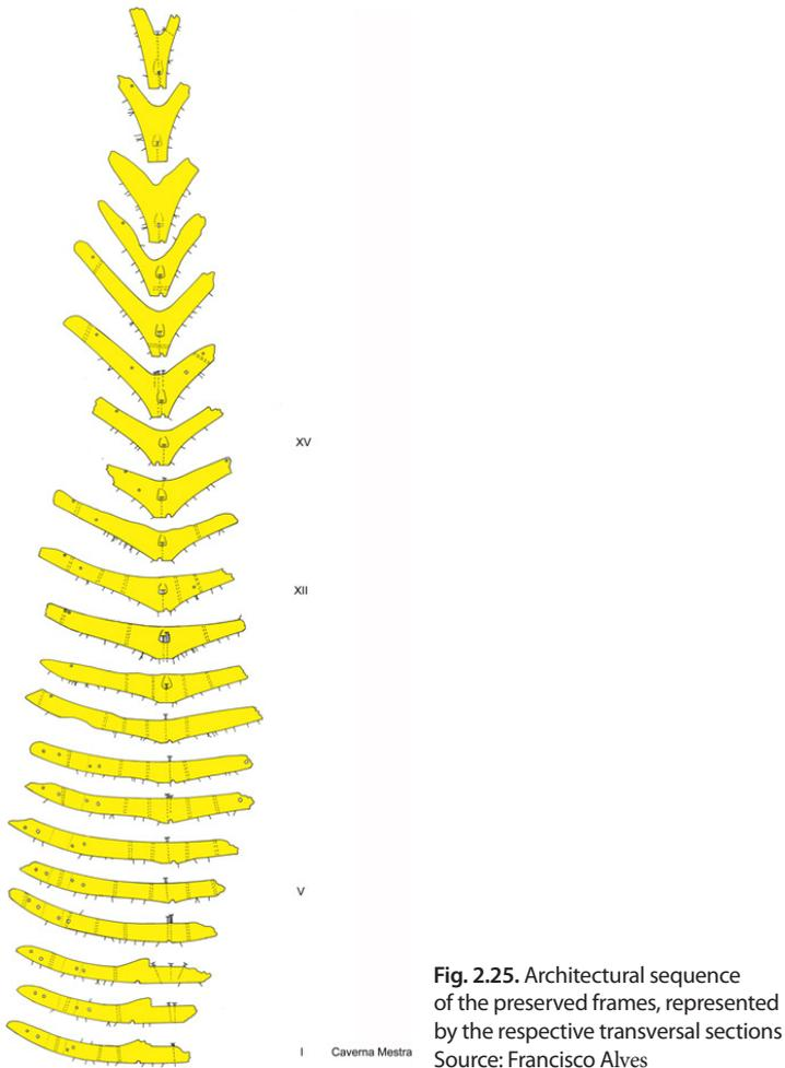
**Fig. 2.25.** Architectural sequence of the preserved frames, represented by the respective transversal sections
