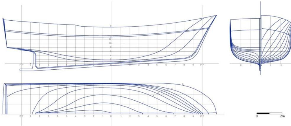
Fig. 3.1. Geometrical plane of the hull planking exterior
