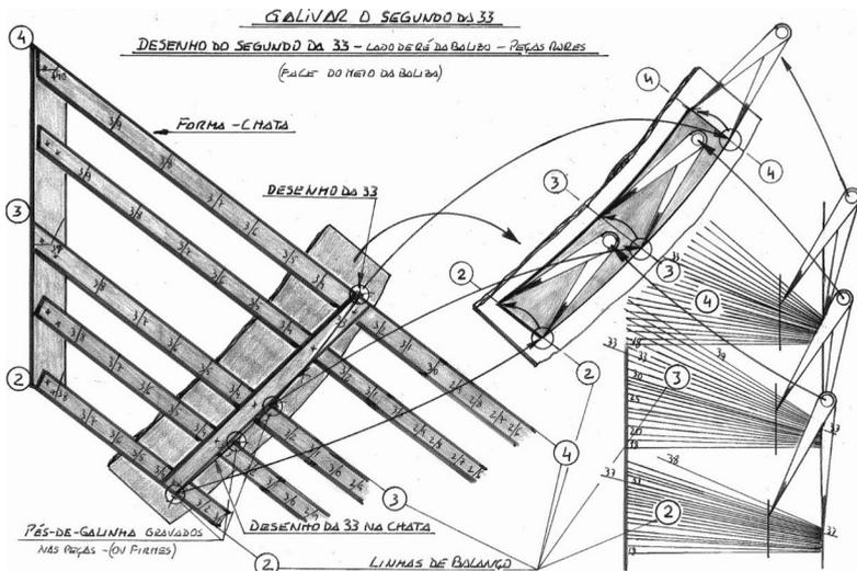
Fig. 3.21. Wood shaping the second of frame 33
