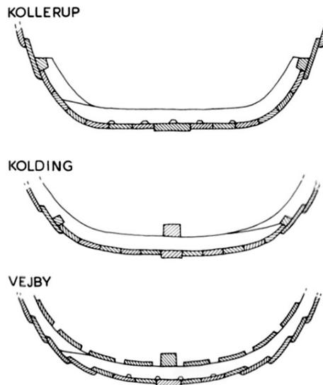
Fig. 2.32. Central sections of the cogs from Kollerup, Kolding and Vejby
