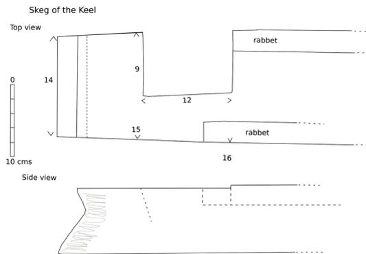
**Fig. 1.6.** The open mortise in the aft extremity of the keel
