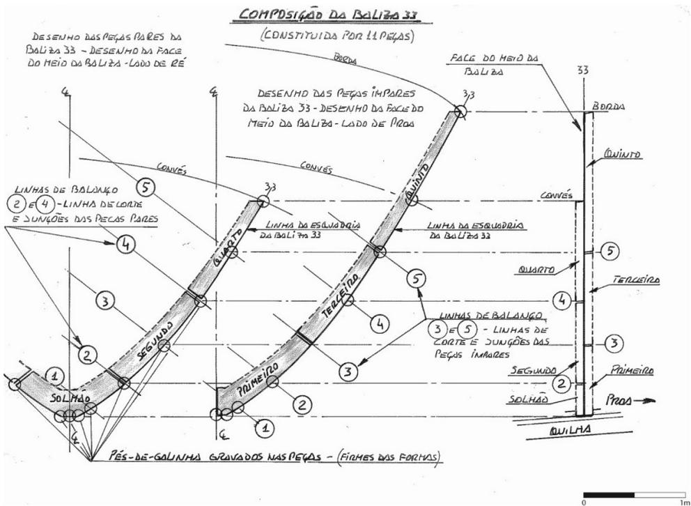
Fig. 3.13. Section in the middle of the frame, dividing the odd and even parts
