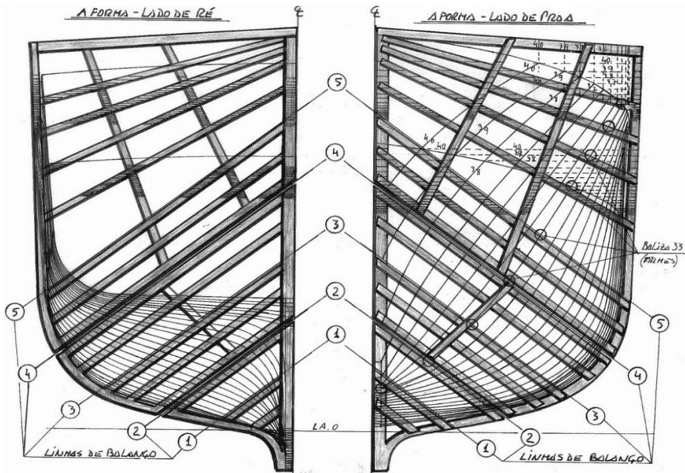
Fig. 3.10. Moulds for wood shaping the frames
