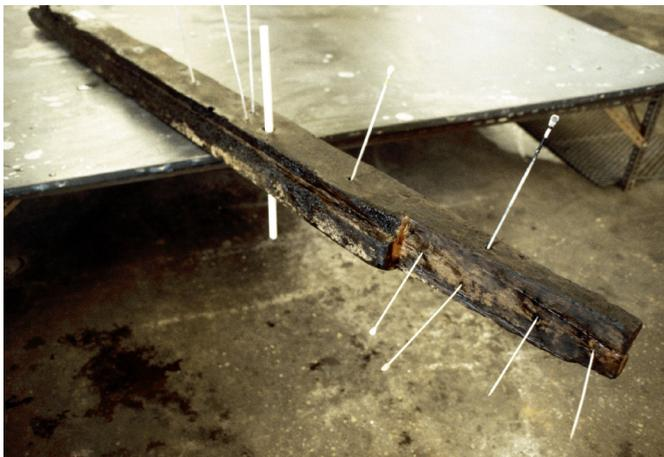
Fig. 2.10. Segment from the keel of *Ria de Aveiro A* with vertical scarfs in their extremities
