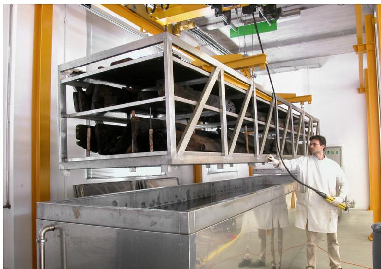
Fig. 2.44. Steel shelf-stand, hanging from a crane, for the immersion of the wooden structural pieces of RAVA. It could be moved, longitudinally and transversally, over the tanks' area, by means of a «chariot» with manual control working on rails supported by an iron structure composed with H-shaped girders, anchored to the concrete pillars of the building
