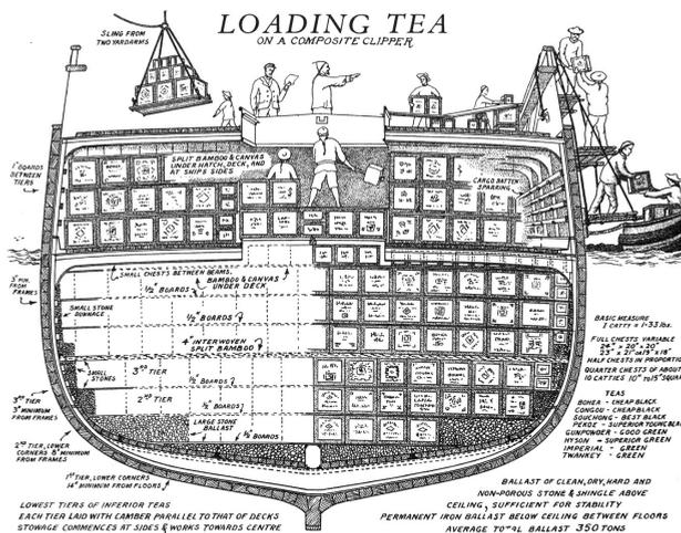
Fig 8.8. Loading tea in tea-chipper in China drawings of *Cutty Sark* sales and rigging
