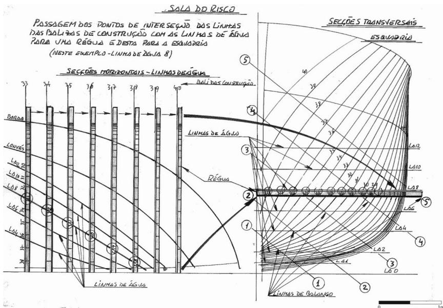
Fig. 3.5. The process of obtaining the plane of transversal sections
