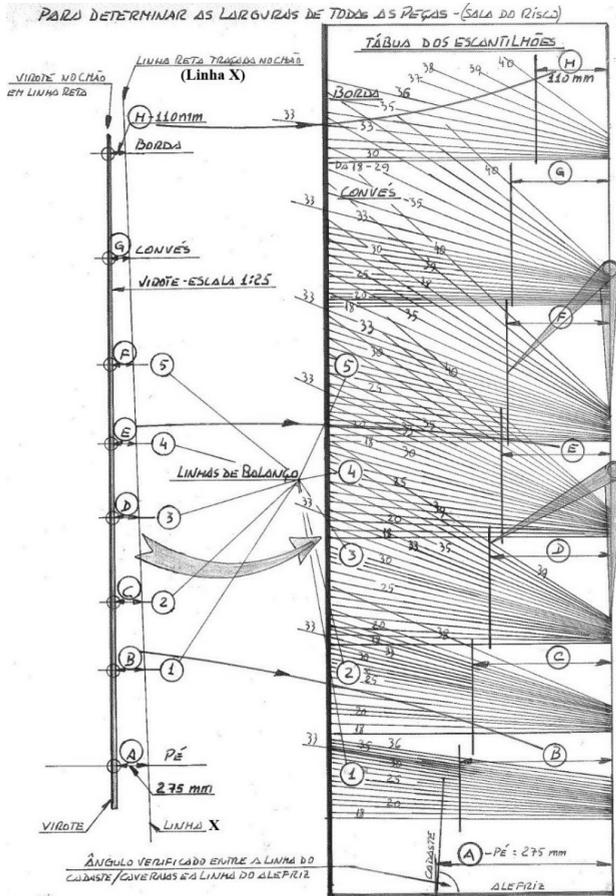
Fig. 3.9. Transposing the widths from the spline to the wooden board (2nd step)
