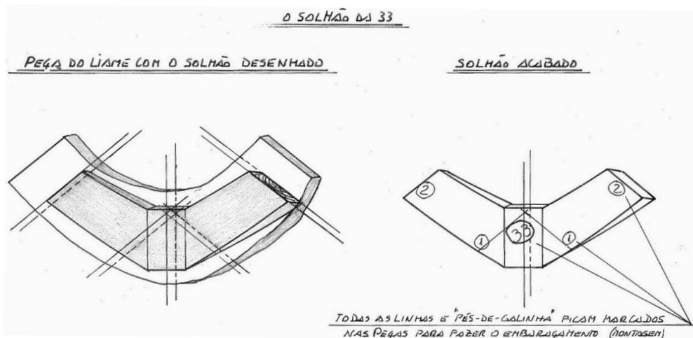
Fig. 3.19. The completed floor timber
