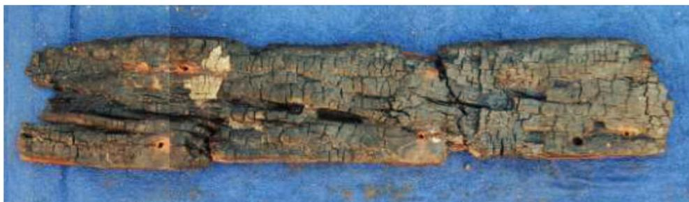
**Fig. 2.18.** Fragment of a starboard side hull plank burnt on its internal face
