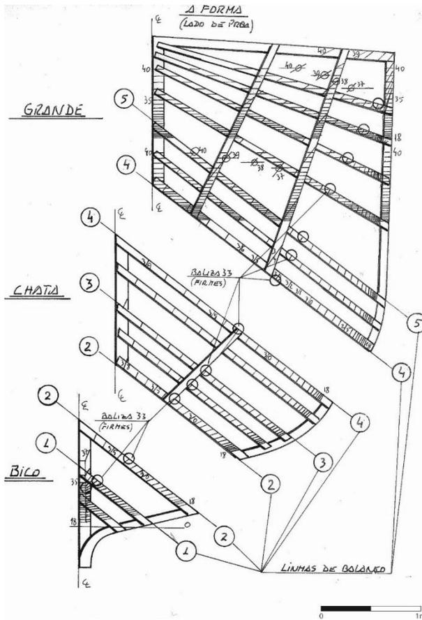
Fig. 3.11. Moulds for wood shaping the frames, apart
