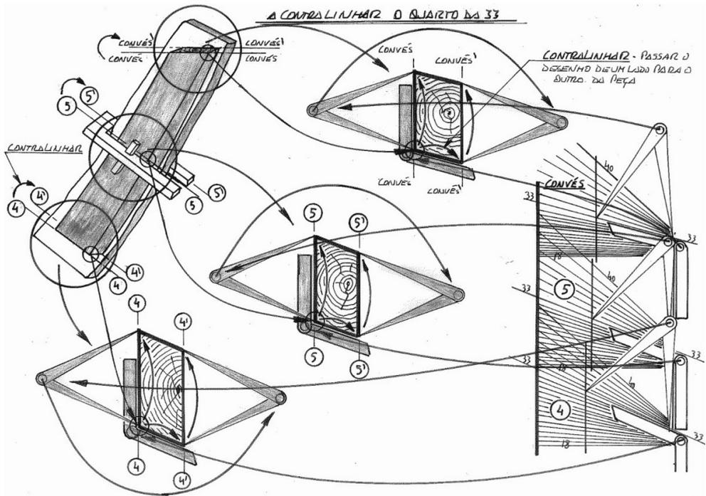
Fig 3.24. Counterdrawing the fourth of frame 33
