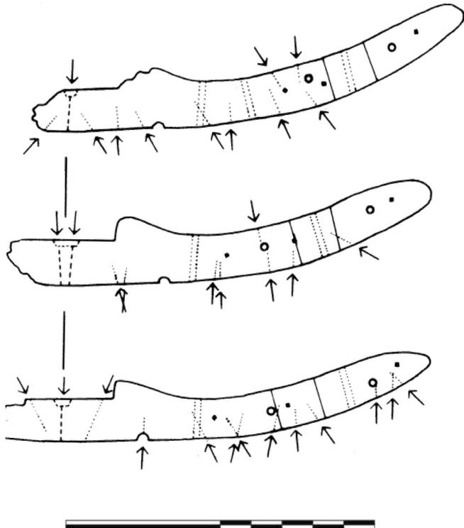
Fig. 2.20. Drawing of the axial-transversal sections of the first three partially preserved frames
