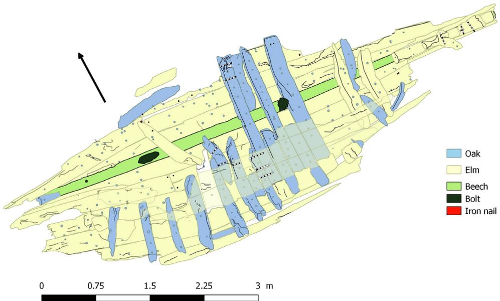
Fig. 1.14. Planimetric view of the various wood species in relation with the architectural remains
