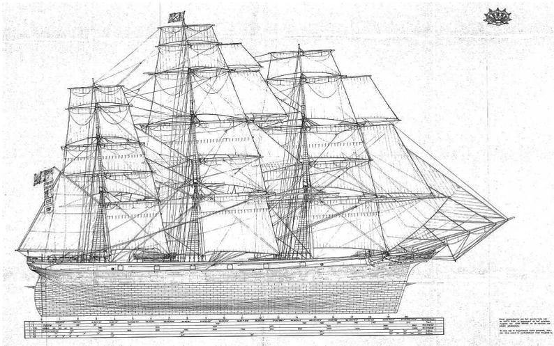
Fig 8.9. Drawings of *Cutty Sark* sails and rigging
