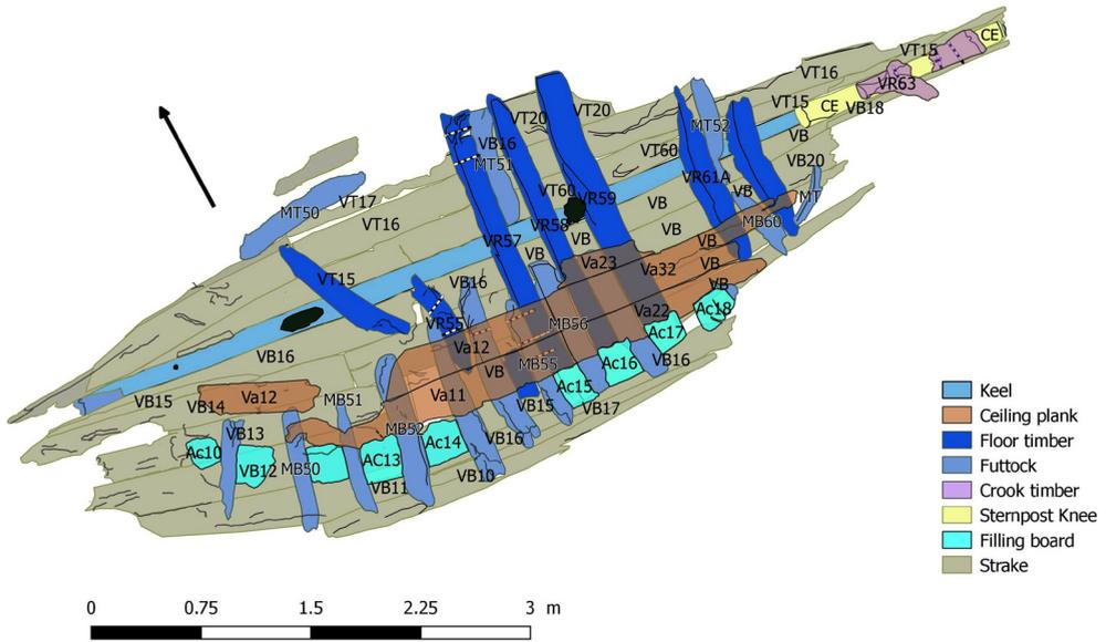
Fig. 1.4. Identification of the architectural elements
