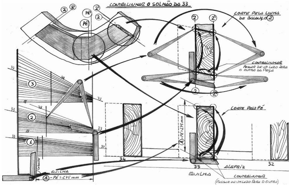
Fig. 3.18. Counterdrawing the floor timber of frame 33
