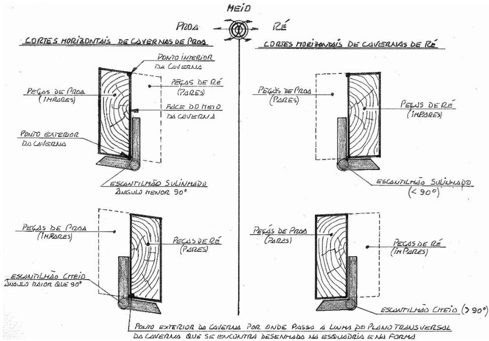
Fig. 3.15. Obtuse slope angles and acute slope angles
