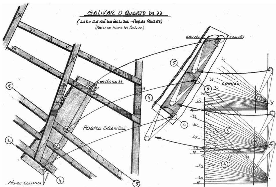
Fig. 3.23. Wood shaping the fourth of frame 33
