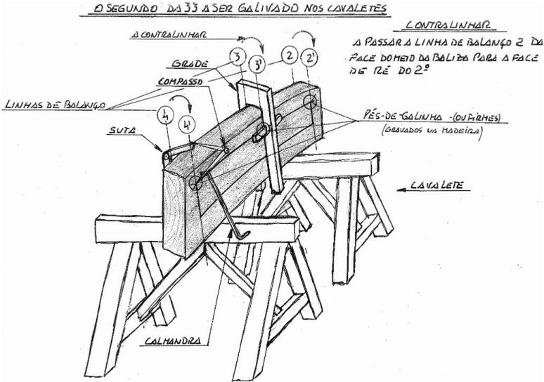
Fig. 3.20. Wood shaping the second of frame 33 at the easels
