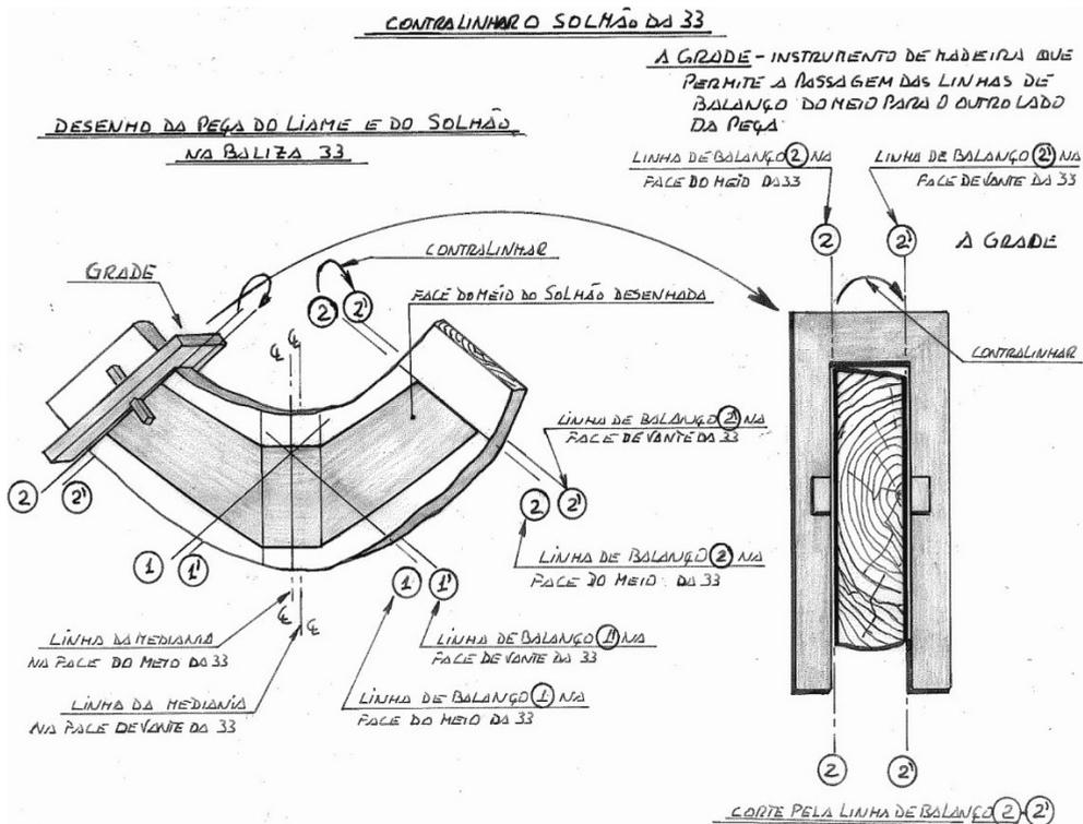
Fig. 3.17. Counterdrawing — Image of the counterdrawing grid
