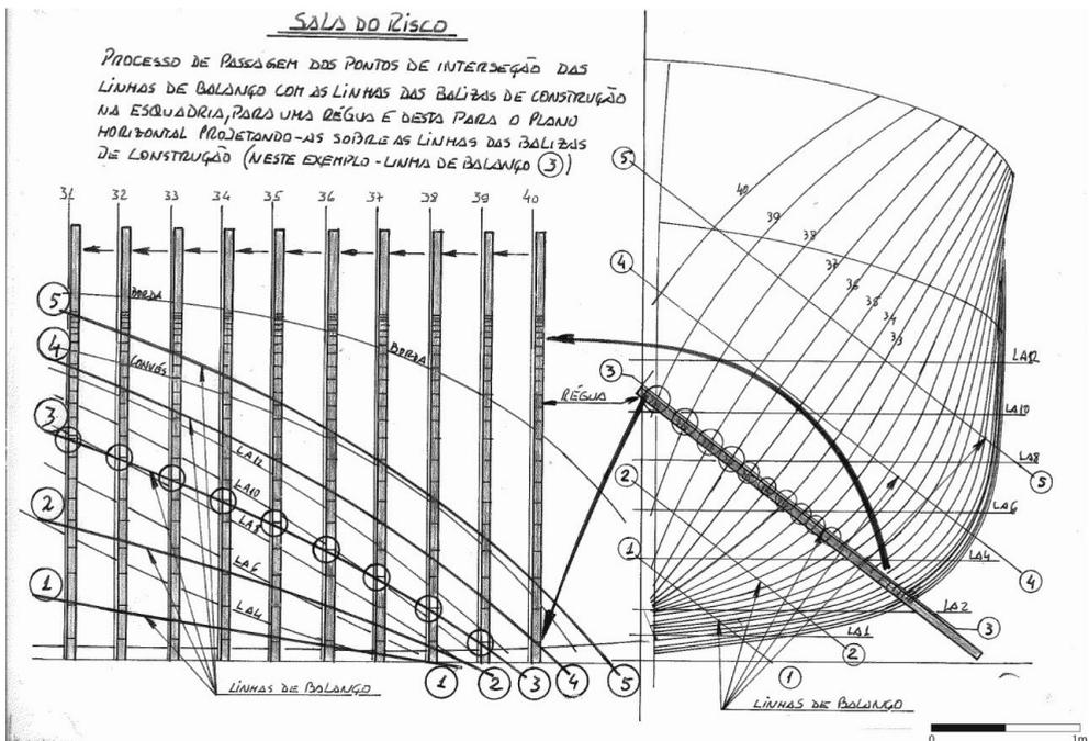
Fig. 3.6. Horizontal projection of balance lines
