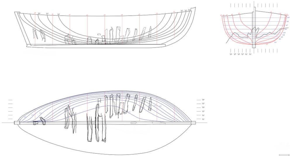
Fig. 1.16. Reconstruction of the lines
