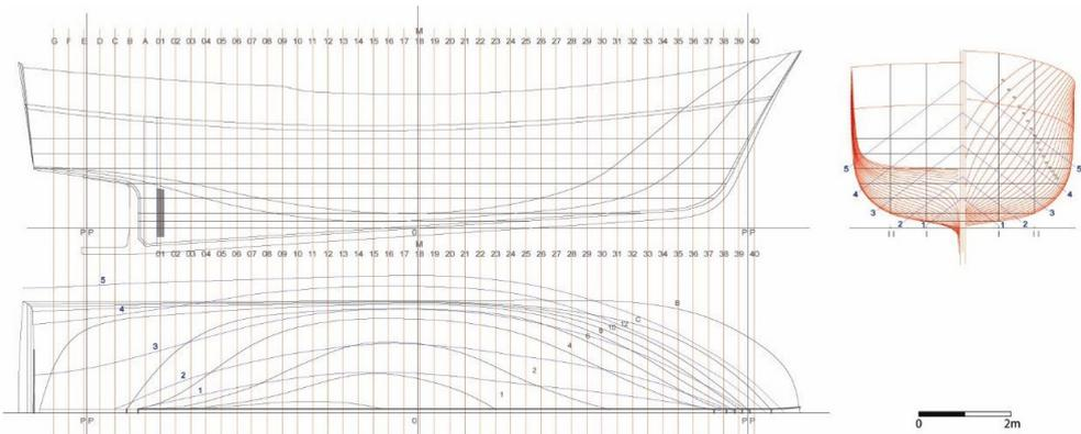
Fig. 3.4. Division and marking of the 40 frame lines
