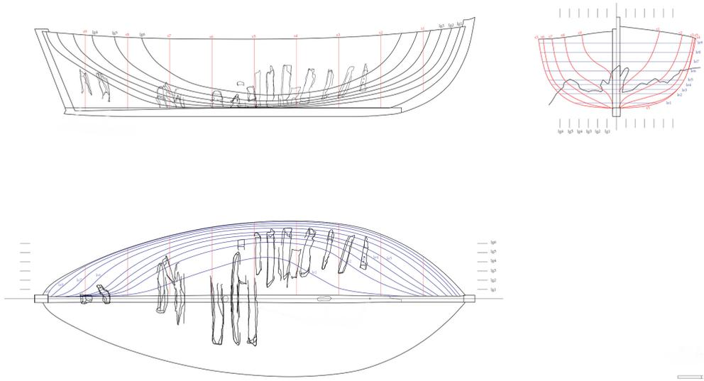
Fig. 1.16. Reconstruction of the lines
