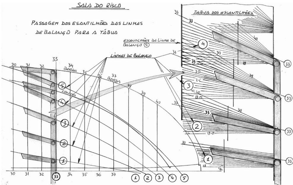
Fig. 3.7. Transferring from the balance lines slope angles to the slope angles' wooden board, between the 30th and the 40th frames
