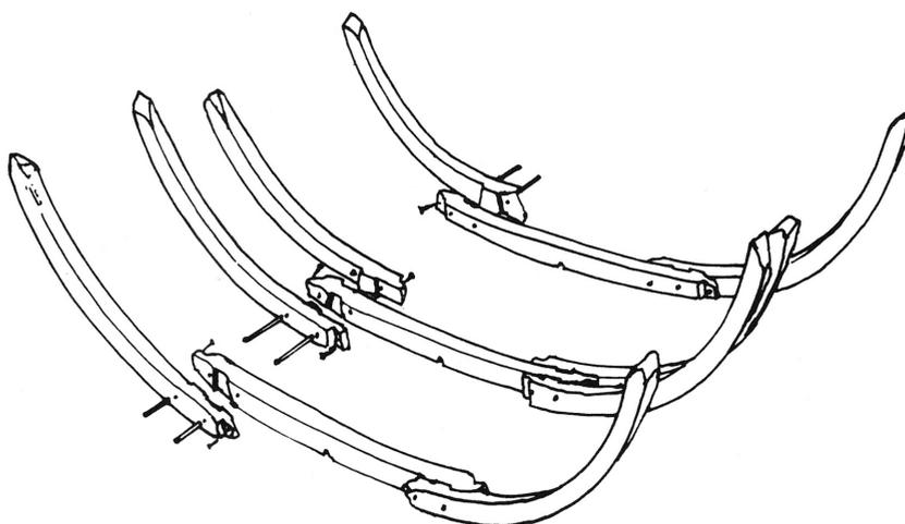
Fig. 2.14. The so-called Atlantic scheme of the master-frame and its adjacent frames
