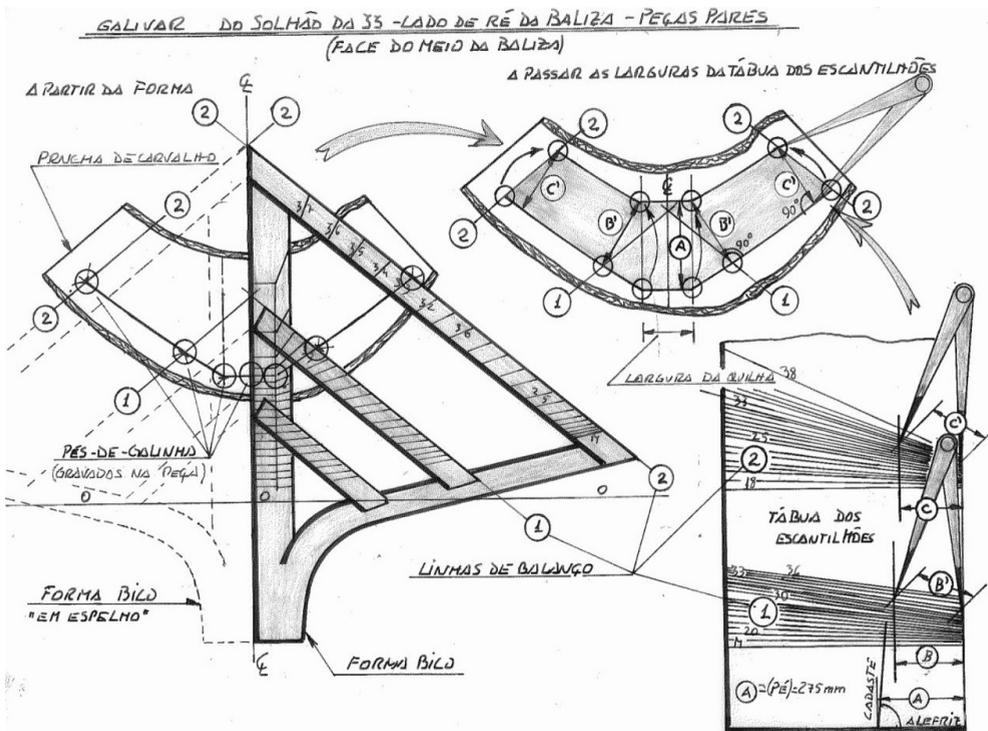
Fig. 3.16. Wood shaping the floor timber of frame 33
