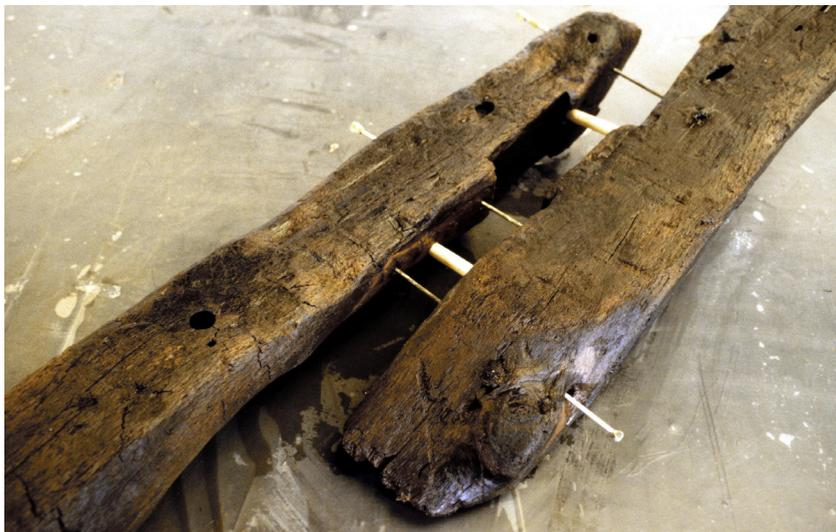
Fig. 2.13. Typical frame-futtock connection, through dovetail mortise and double fastening, with iron nails and wooden pegs
