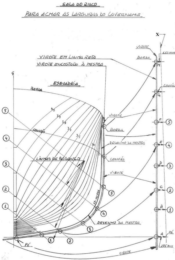
**Fig. 3.8.** Width extraction to the spline (1st step)
