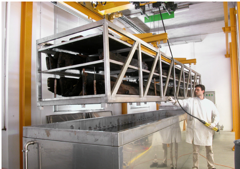
Fig. 2.44. Steel shelf-stand, hanging from a crane, for the immersion of the wooden structural pieces of RAVA. It could be moved, longitudinally and transversally, over the tanks' area, by means of a «chariot» with manual control working on rails supported by an iron structure composed with H-shaped girders, anchored to the concrete pillars of the building Source: Francisco Alves
